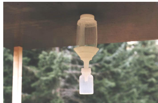
Fig. 2. The surrogate surface that is simple to produce mounted under a roof.
